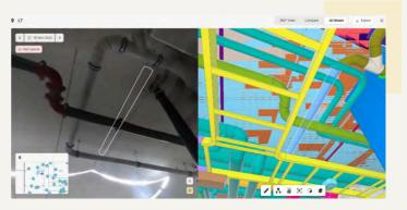
After being alerted of the incorrect positioning of a pipe, Oulu's project teams readjusted the installation before the error could snowball
