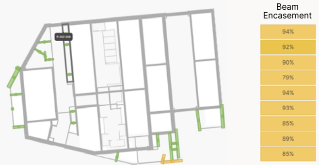
Example of a floor where beam encasement capped at approximately 90% completion.
